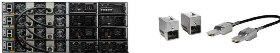
Figure 4. StackWise-160 Kit with Stack Adapters and Cables
